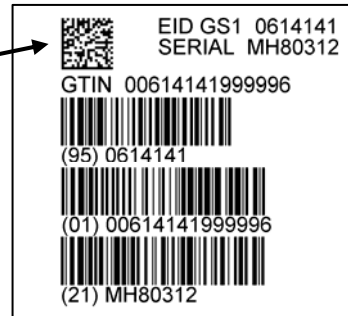
FIGURE 7. Example GS1 label (equivalent UII in UCC/EAN-128 and Data Matrix).
