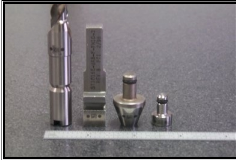
Example production tools laser marked with a Data Matrix code.
